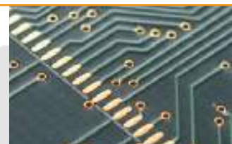
Measuring PCBs: Au/Ni/Cu/PCB
