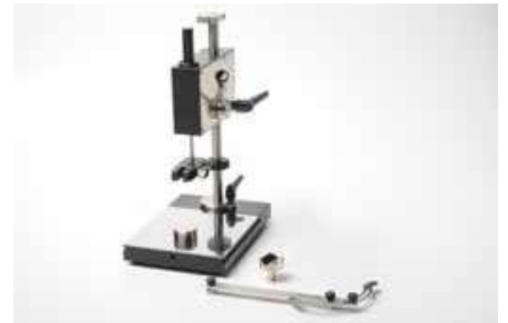
Stand for clamping internal probes
