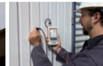
Measurement of a paint coating on steel
